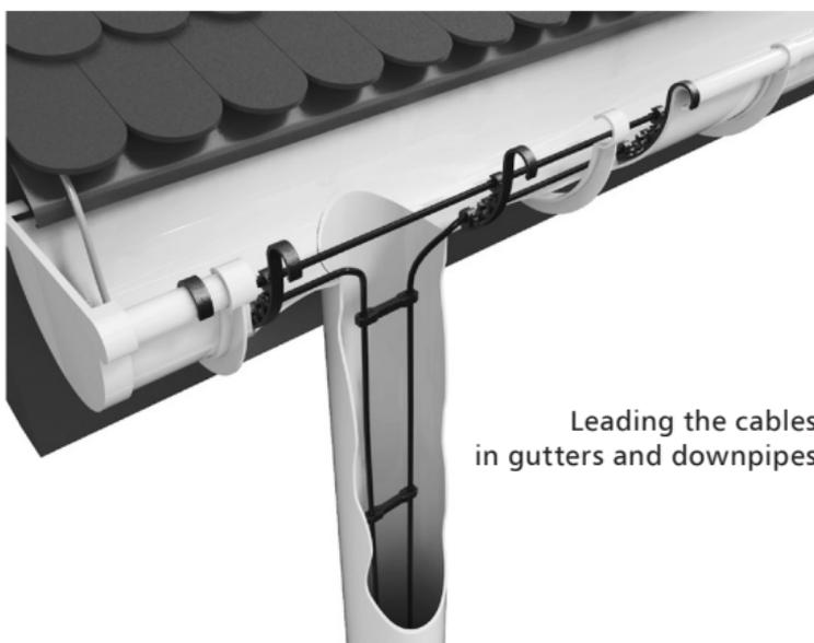
Leading the cables in gutters and downpipes
